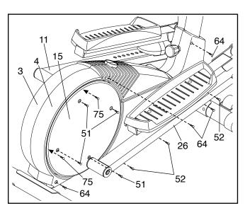
Next, remove the four Screws (51) from the right Pedal Disc (15), and slide the Pedal Disc off. Remove all Screws (52, 64) from the Right Side Shield (4) and the two Bolts (75) from beneath the Pedal Disc, and remove the Right Side Shield (4). Remove all Screws (52) from the Left Side Shield (3) and remove the Left Side Shield.
